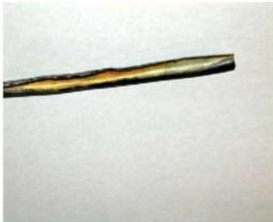
After 30 cycles with peracetic acid and no mechanical support
