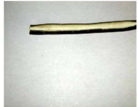
After 30 cycles with peracetic acid and with mechanical support
