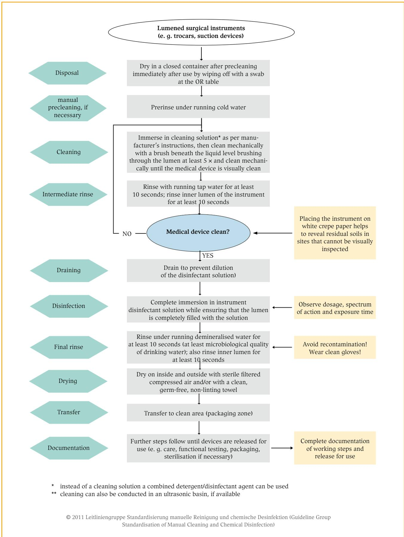
Fig. 2: Flow chart: Surgical instruments with lumen
